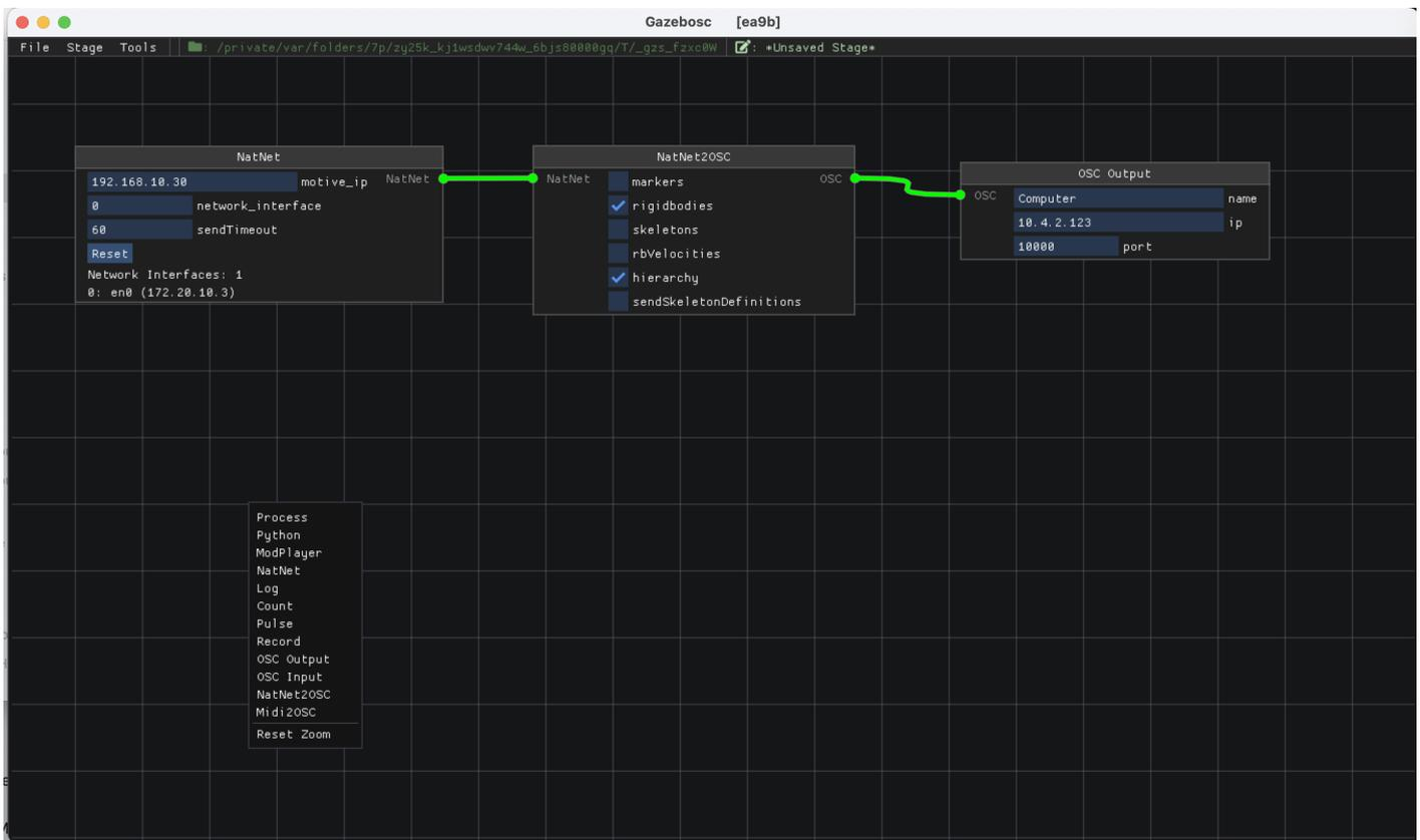
Once the correct connection is established between Motive and Gazebo the patch cords connecting the actors should colour green, an indication that data is streaming through Gazebo. To monitor the OSC data from GazeboOSC, or other OSC, data you can download the free OSC and MIDI monitoring application [Protokol](#).
