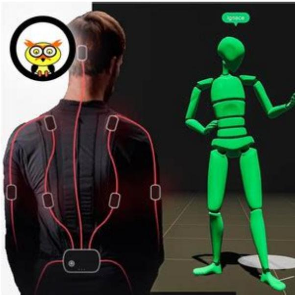
The **Rokoko SmartSuit Pro** is a **wireless motion capture suit** that tracks full-body movement in real time. It's made up of sensors placed around the body, allowing you to **capture the motion of a performer** and translate it into digital animations..
