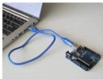
Connect your Arduino board to the host computer.
