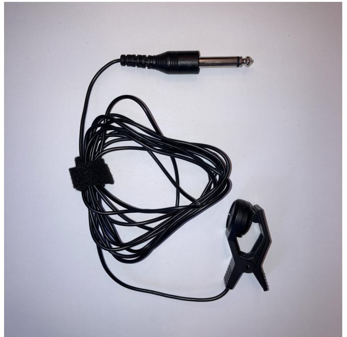
(fig.2 ) piëzo-electric microphone with integrated clamp.
