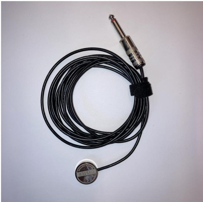
(fig.1 )piëzo-electric microphone in metal housing.
