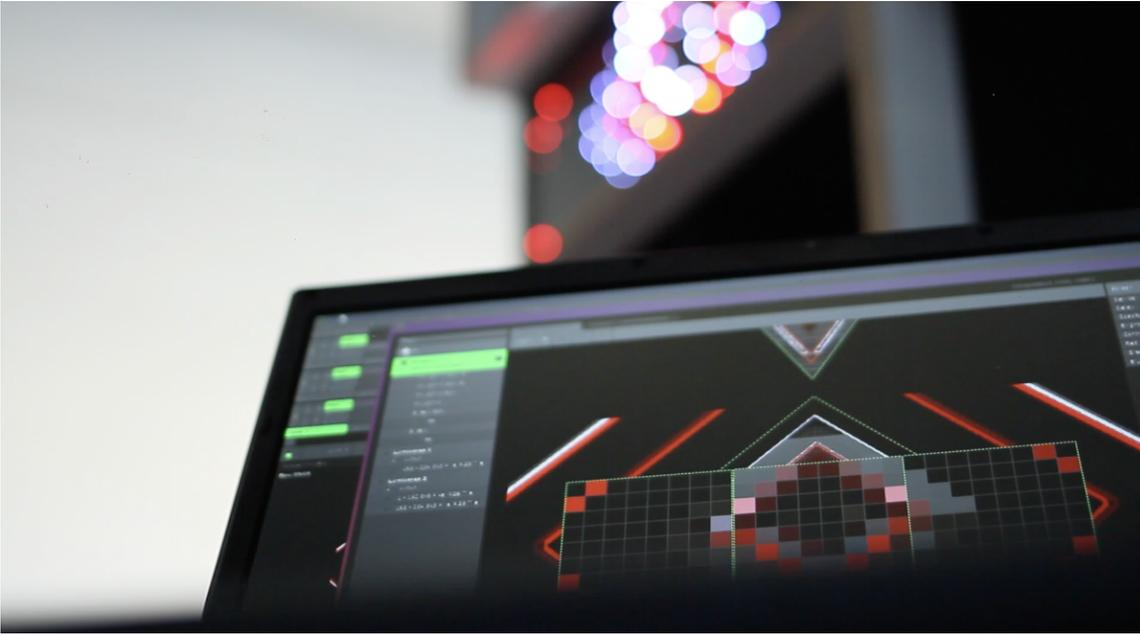
**Resolume Arena** is Vj software, normally used for sending visuals to screens. But can also can output the color or brightness of your pixels to LED strips or other light fixtures via DMX. Beware that you need a hardware controller to covert you signal to DMX, NOT an Enttec..... ([see below](#))
