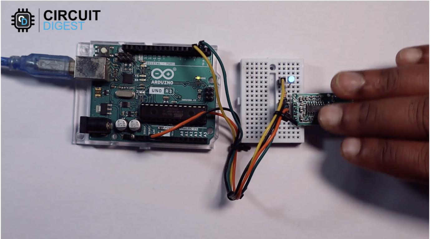
And a tutorial explaining the RCWL-0516 Microwave Doppler Radar sensor and running a beginner test can be found [here by CircuitDigest](#) .
